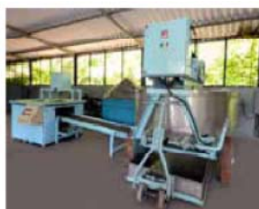
photo 1 UMMB plant with pneumatically controlled rotary pressing device for UMMB feeding to animals
