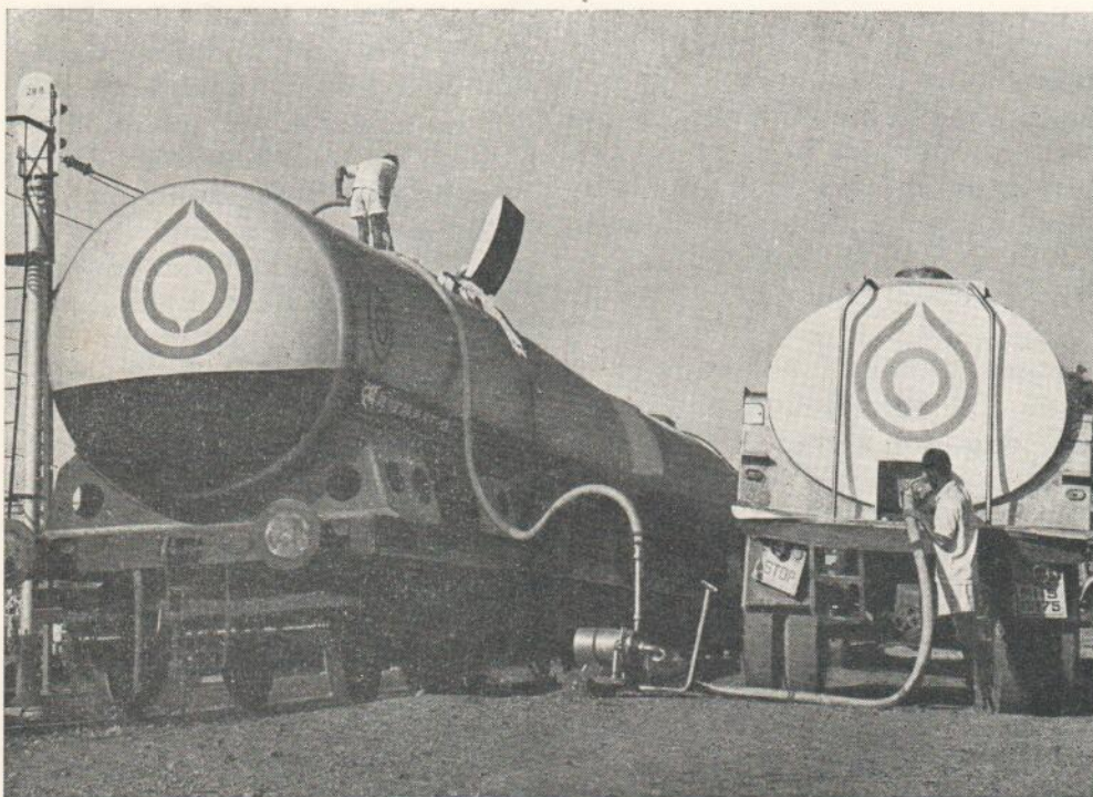
Specially built, insulated rail and road tankers transport the milk to distant cities.
