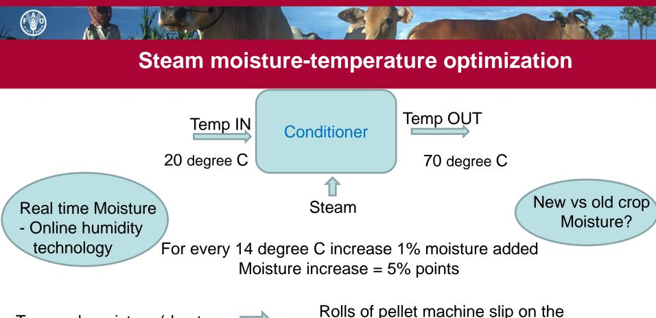
Too much moisture (due to excess steam) to feed mesh
