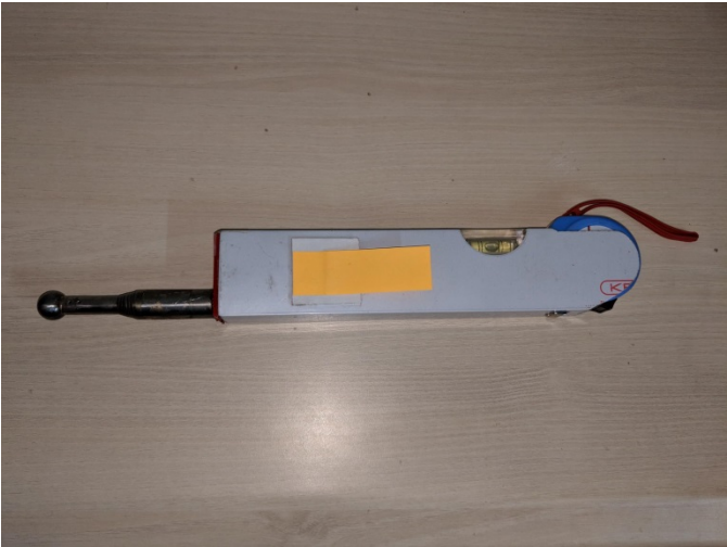
Figure 2: Retractable measuring tape with levelling bubble and telescoping rod-like attachment
