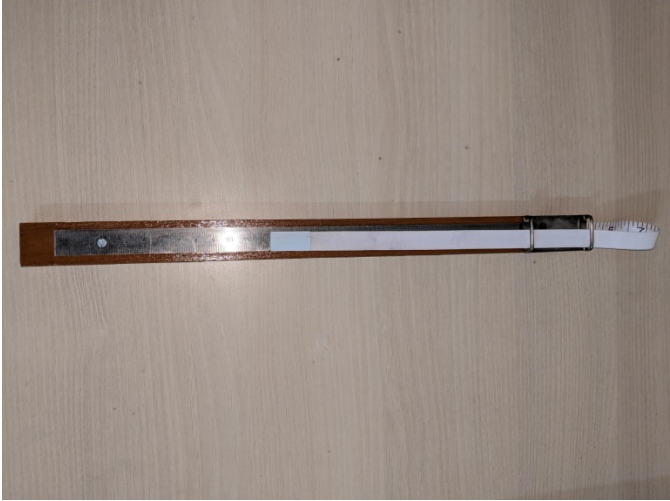
Figure 3: Circumference measuring device
