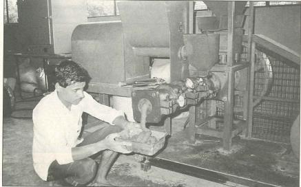
Using an extruder for the manufacture of block
