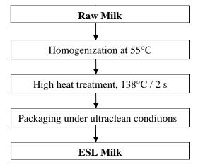
Figure 1: ESL process - High heat treatment
